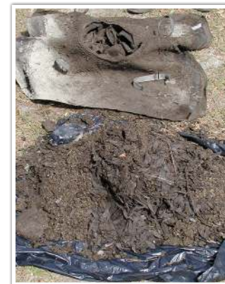
Actual Drain Guard test unit - over 50 lbs. of sediment removed.
