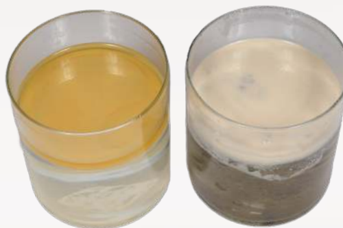
Test samples: Container on left shows untreated oil and water. Container on right was treated with Ultra-Archaea and shows that only lipids were left after the bio-remediation took place. The dark material in the bottom of the container is the clay carrier.
