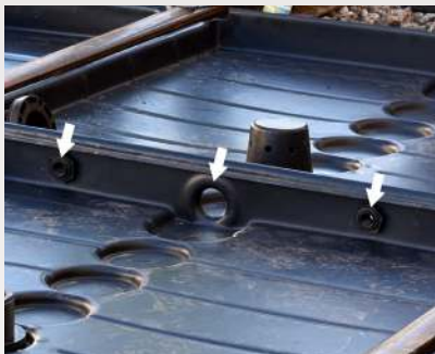
Flow-through channels — All Pans are connected "end-to-end" with bulkhead fittings, and a 3-inch diameter flow-through channel, allowing spills to quickly travel from one Pan to the next.
