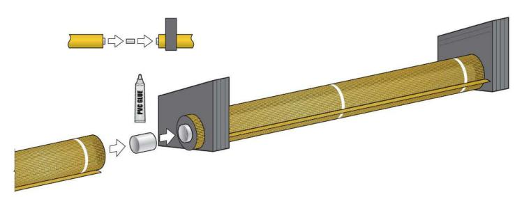
3. Once the two sections are connected together, slide the Anchoring Wedge to cover and seal off the seam area between the two sections.
