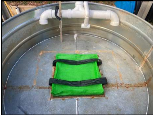
Product Installed / Grate In Place / Test Initiated
