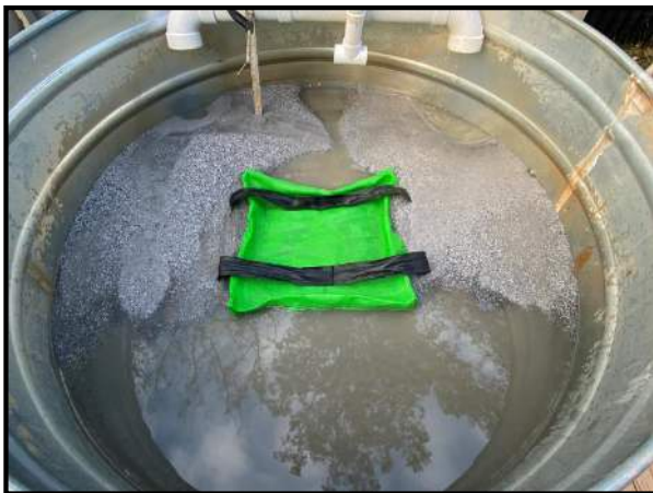
Deposition At End-of-Flow / Close-up of Captured Sediment
