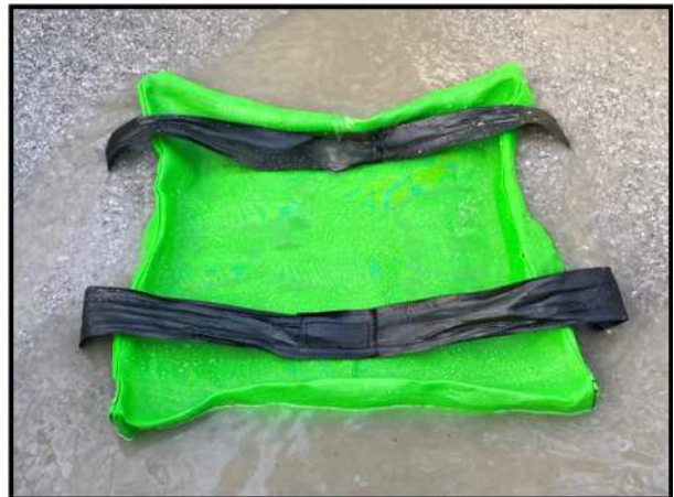
Deposition At End-of-Flow / Close-up of Captured Sediment
