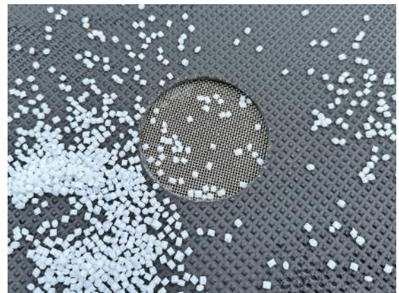
Mesh drain allows liquids from contained spills or water from rain to pass through while capturing plastic pellets.
