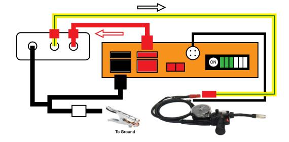
**WARNING:** Connections should mirror the wiring diagram. Wrong connections will cause the controller to be inoperable. Double check connections before turning the unit on.
