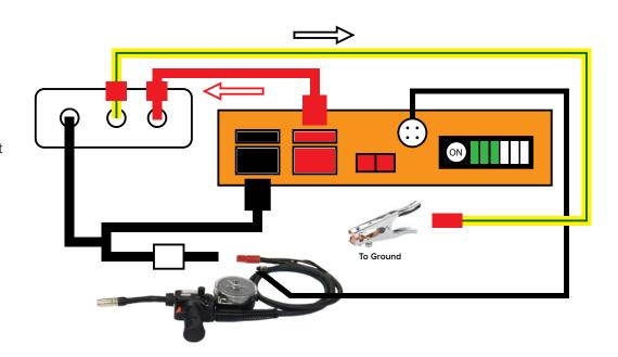
**NOTE:** To weld with flux core wire using the reverse polarity configuration, connect the yellow/green wire from the amperage controller to the ground clamp, and one of the black cables from the amperage controller to the red Anderson connector on the gun.
