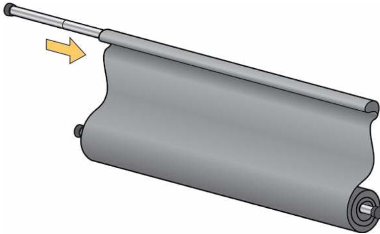
**Step 6:** When you insert the rods into the curb inlet opening, pinch the 2" of excess filter material at each end of the tension rods between the end of the rod and the wall of the opening. This will keep the Filter Insert tight and help seal off the edges. On the bottom tension rod you only need to secure a single layer of filter material between the end of the rod and the wall of the opening.
