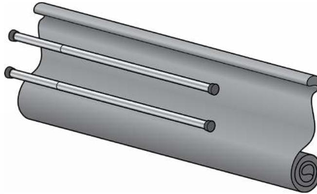
**Step 2:** Measure the opening of the curb inlet at the point where the Tension rods will be placed at the top and bottom of the inlet opening. The top tension will be placed 1" from the top of the opening to allow emergency overflow in a flood-type situation. The bottom rod will be placed against the bottom of the opening. For both the top and bottom tension rod, they should be placed in the inlet opening so they will be flush with the curb face when installed.
