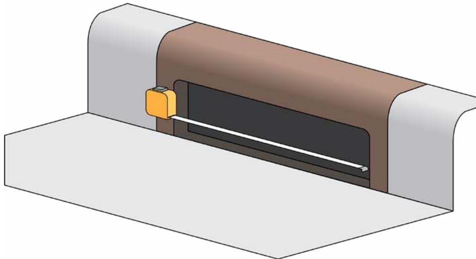
**Step 3:** Lengthen or shorten each tension rod to be approximately  $\frac{1}{2}$ "-1" longer than the dimension you measured in Step 2. This will allow you to compress the spring in the tension rod as you insert it to assure a tight and secure fit.
