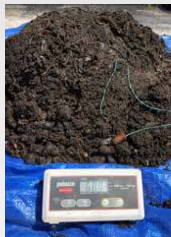
Actual drain guard test unit — over 50 lbs. of sediment removed.
