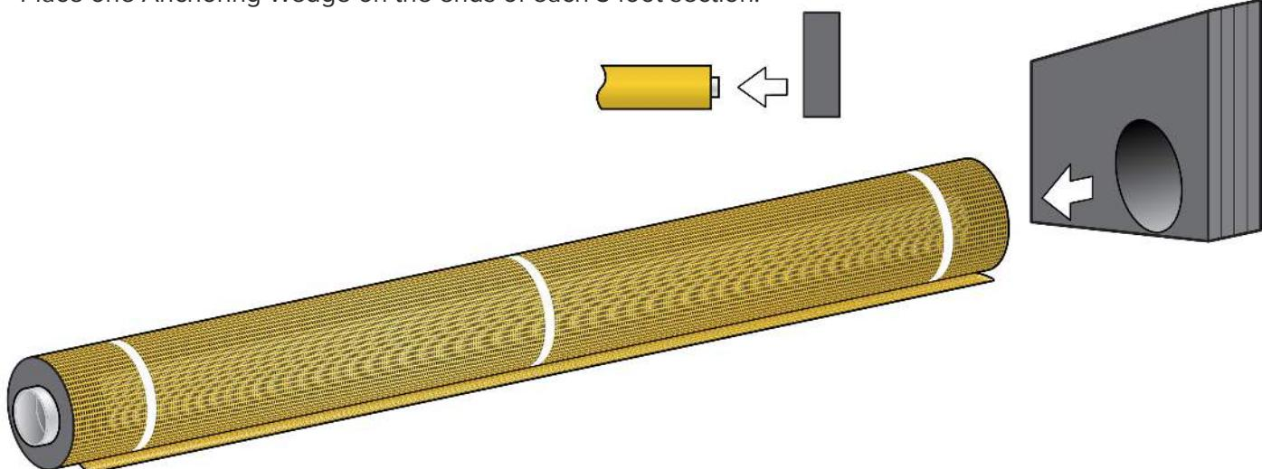
2. Connect together two sections of the CurbGuard Plus by inserting the Male Pipe Connector into the open end of the Female Pipe Fitting. (gluing the sections together using PVC cement is optional)
