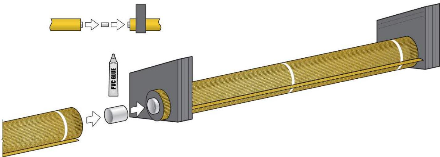
3. Once the two sections are connected together, slide the Anchoring Wedge to cover and seal off the seam area between the two sections.
