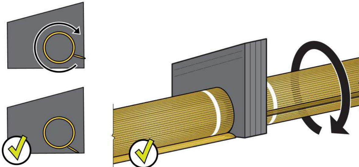
5. Install the assembled unit into the “throat” of the curb inlet by pushing each Anchoring Wedge down into proper position (Note: The black corrugated plastic covered part of the Wedge should face down—toward the ground) . At the ends of the curb inlet, position the Anchoring Wedges to seal off the corners.
