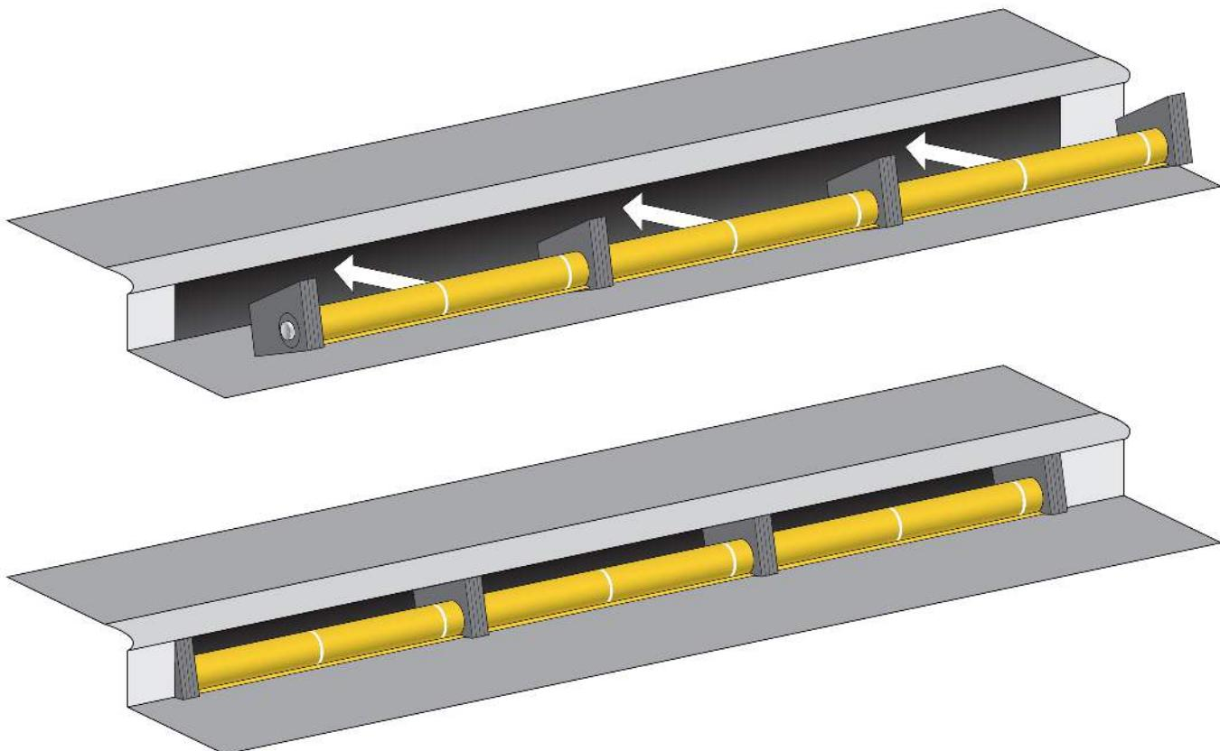
+ Note: The top of each Anchoring Wedge is perforated. If the Wedge is too large for the inlet, simply tear off the top section and reinstall (a second perforation is available if needed). The front of the Anchoring Wedges should be flush with the face of the inlet.
