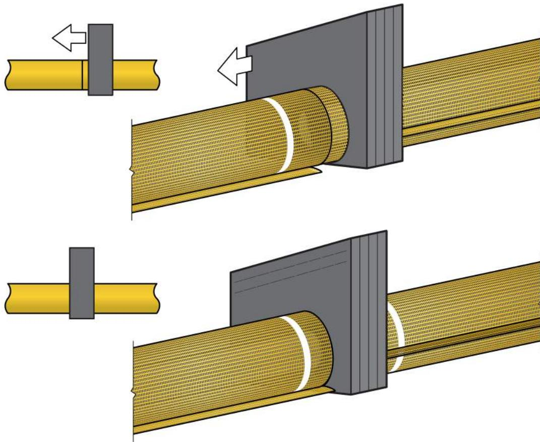
4. Align the CurbGuard Plus with the Sediment Flap facing down (to touch the pavement). This will form a barrier against water flowing underneath the unit and will prevent water/sediment bypass.
