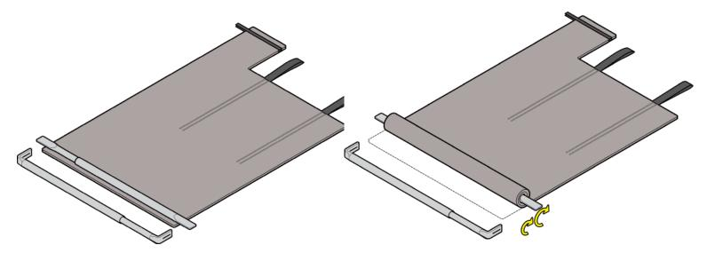
Step 1: Place the straight bar (flat ends) and locking bar (90 degree bend at both ends) at opposite end from hose opening.
