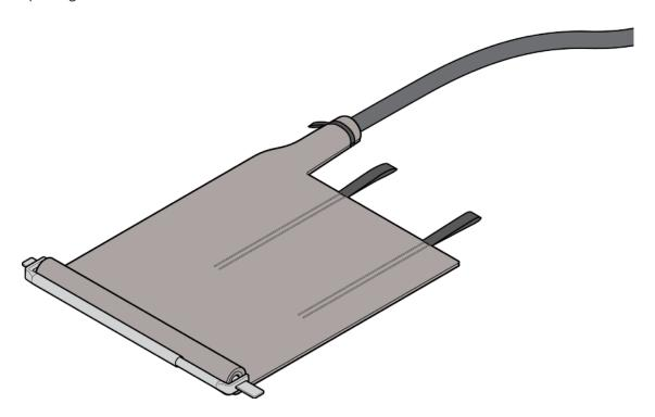
Step 3: Place flat ends of Straight Bar through slots in ends of Locking Bar and adjust to width of Dewatering Bag. Unit is now ready for use.
