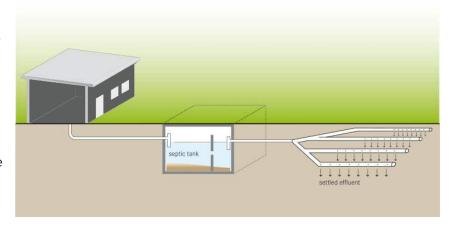
water-soluble fatty acids, carbon dioxide and water. Water exits the tank below the floating material and above the settling solids. The water flows to the leaching field. Sludge builds up in the septic tank and the tank must be pumped periodically; if not, scum may overflow into the leaching field.
