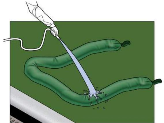
**STEP 3:** Place the Ultra-Filter Sock across the opening of a curb style catch basin or in front of a grated catch basin where stormwater flows into the catch basin. Use the Ultra-Filter Sock to intercept the stormwater flowing into the catch basin and allow the stormwater to flow through the sock's filter media to help remove the heavy metal pollutants.
