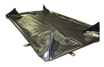
3. Slide L-brackets into the Berm pockets to support the sidewalls. Do this for all but the one wall that will be used to load the spill pallet and IBC. (NOTE: the longer (17") side of the bracket should be inserted into the sleeve. The shorter (11") side will go
