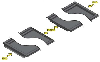
2. It is important to install the center track pans so that they are centered between the two rails. This will facilitate the installation of the center track pan gaskets at the end of this process. In order to keep them centered UltraTech recommends cutting four blocks of quarterboard (5/4) wood 6 inches long. These blocks are to be used as spacers to keep the center track pans centered between the two rails while assembling.
