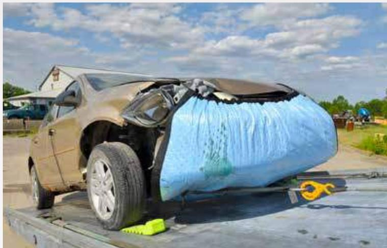
Ultra-Spill Diaper being used to contain fluid spill from wrecked vehicle
