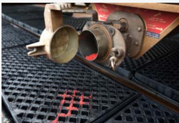
Included grating allows pellets to pass through - provides safe walking surface
